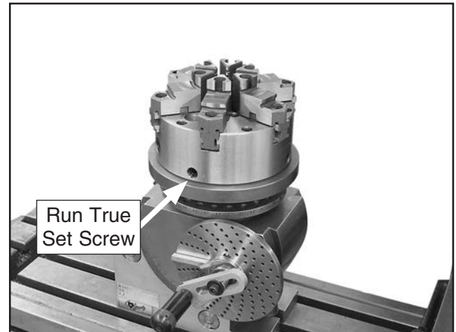
Figure 18. Model G9856 6-jaw run true chuck installed (Model G1054 only).
