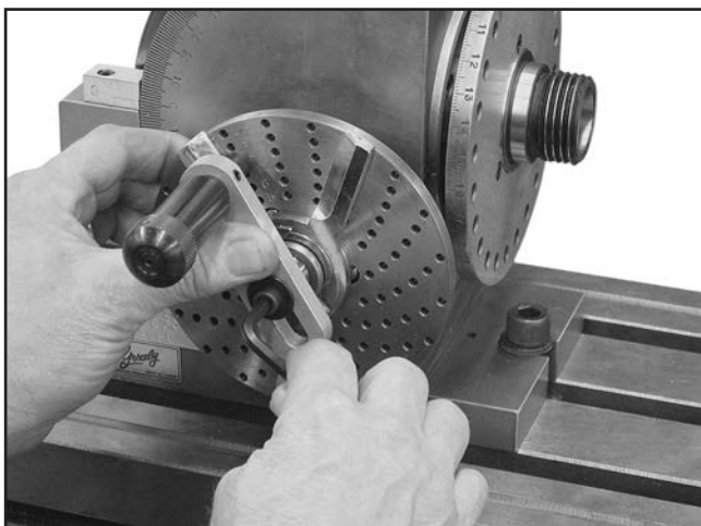
Figure 20. Adjusting the position of the crank index pin.
